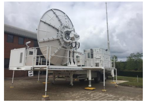
6.3m antenna on trailer mount
