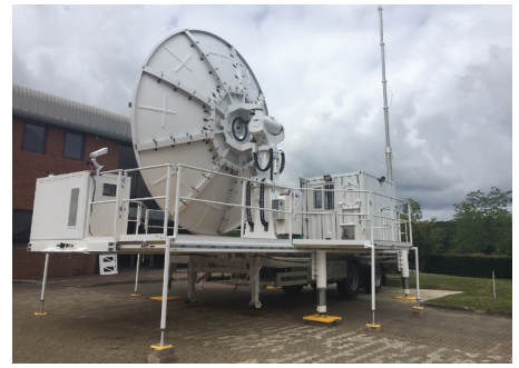
6.3m antenna on trailer mount
