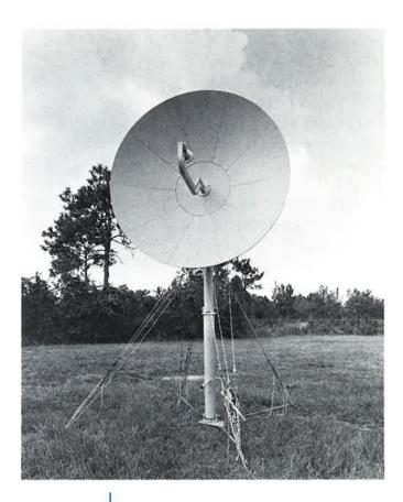
Comtech Antenna Systems, Inc. offers to the troposcatter communications industry this compact, transportable antenna package that provides fast deployment by a maximum of two persons. The reflector measures eight feet in diameter and is constructed of lightweight aluminum. The antenna system operates at a maximum power handling of 5 kilowatts in the frequency range of 4.4 to 5.0 GHz.
