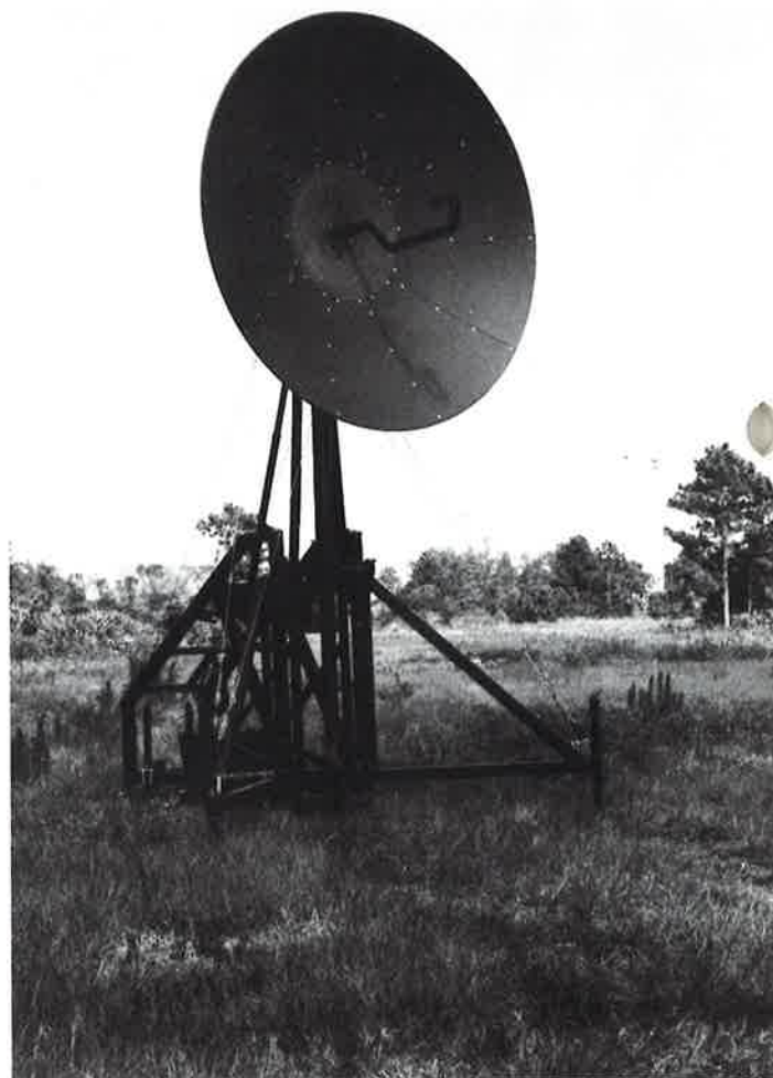
CSI has developed for tactical applications, an eight-foot, highly-compact antenna to provide a means for rapid deployment of troposcatter, line-of-sight or satellite communication systems. The antenna has interchangeable feeds to enable operation in the 4.4 to 5.0 GHz or 7.2 to 8.4 GHz frequency bands. Packed for shipment in a 5 ft. by 5 ft. by 2 ft. container, the antenna can be assembled by one person in less than 15 minutes.
