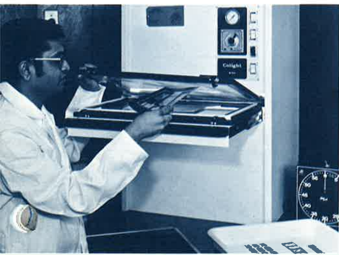
Frame used in the exposure of printed-circuit cards before chemical etching.
